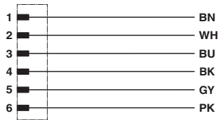
Contact assignment of the M8 plug
